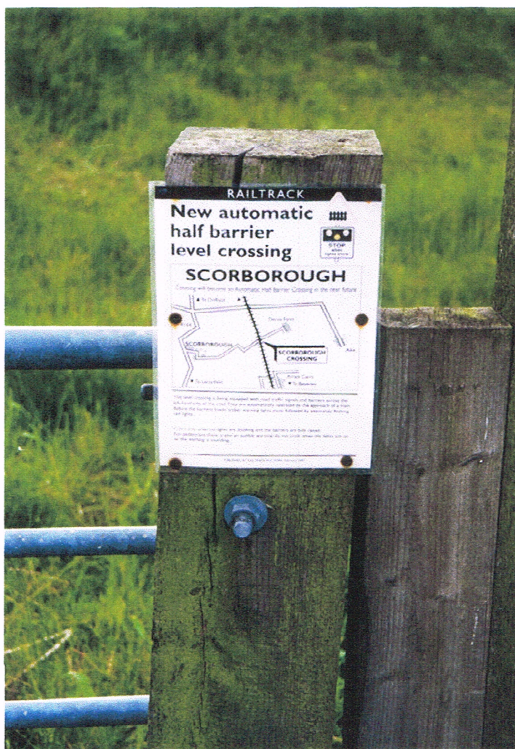
Figure 4.2 Scorborough AHB LC, East Yorkshire; When the LC controls are altered the infrastructure owner has to notify the local people, usually with a leaflet 'drop'. A typical leaflet, in this case plasticised and pinned up at the LC.
