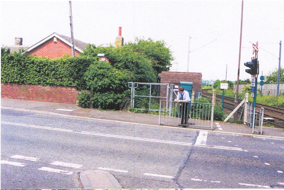
Figure K.13 Bank Foot AOCL LC (top), and Callerton AOCL LC (lh side), TMR; England is a green and pleasant land..... particularly when it comes to obscuring vital road signs with vegetation.
